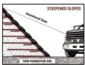
Slopes reinforced with Geotex® geotextiles maximize land use in transportation and site development projects.
